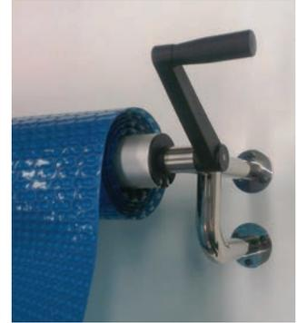
Each system includes a crank handle, a slide-lock anti-unwind device and a fully adjustable cover-to-roller strap kit as standard. The winding crank can be positioned on either end of the reel.
